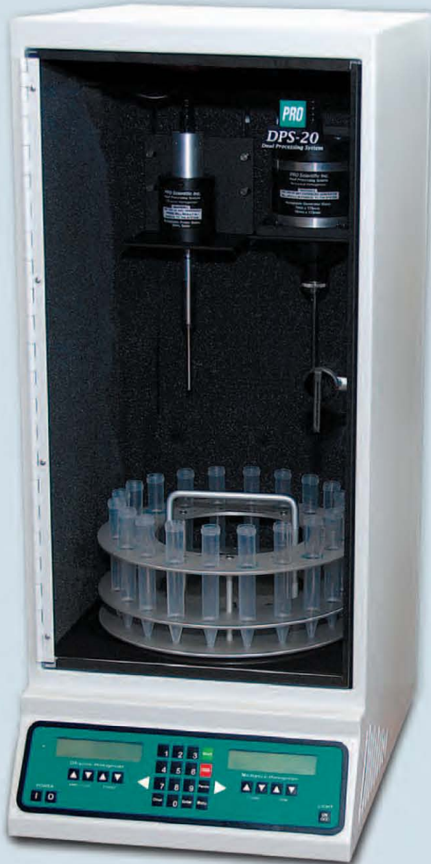
The PRO Scientific DPS-20 shown with 3mm ultrasonic probe, 7x15mm homogenizing generator and 20-space carousel rack for 15ml tubes
