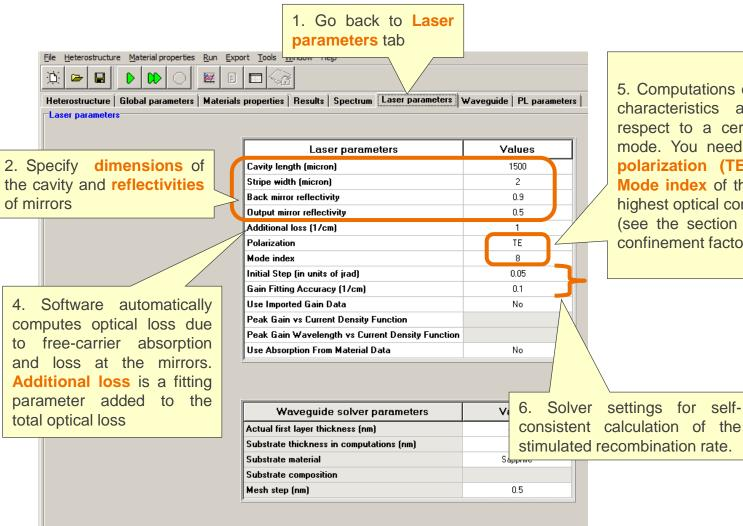
5. Computations of the threshold characteristics are done with respect to a certain waveguide mode. You need to specify the polarization (TE or TM) and Mode index of the mode having highest optical confinement factor (see the section on viewing the confinement factors)
