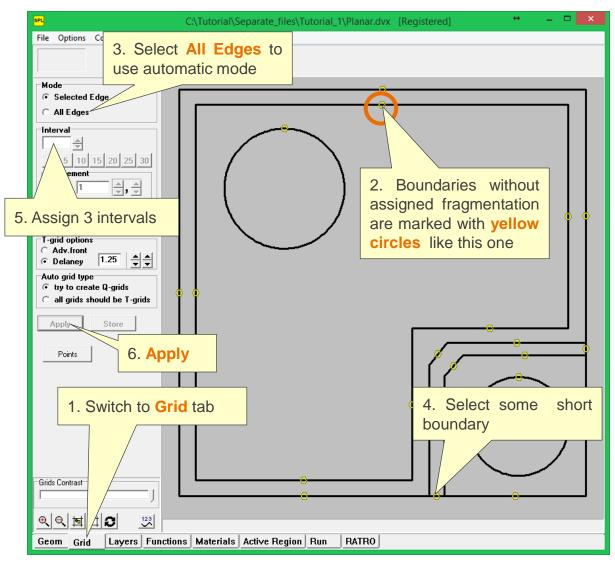
Switch to the tab window Grid to generate the computational grid
