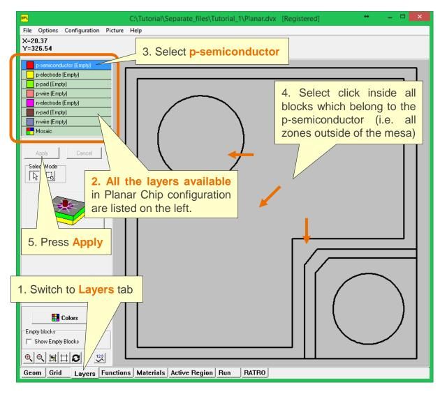
Now the contours are drawn and one needs to convert them into a 3D geometry. You have assigned the thickness of the layer right after the selection of the chip type, but the layers there are listed "by name" (mesa depth, pelectrode, n-pad, etc.) and the software does not know "who is who". Now we will sort it out by establishing connection between outlines and functional elements
