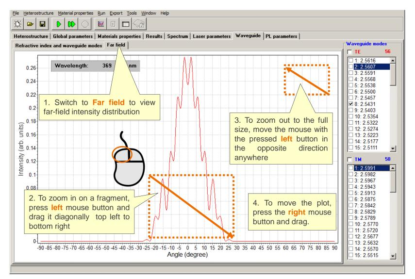
**Tutorial 2: Simulation of InGaN MQW UV laser diode**
