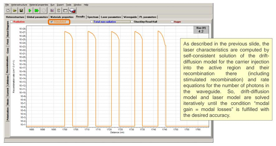
Use Run -> Single Calculation With Laser or Run -> Series Calculation With Laser menu item and specify a bias or a set of biases similarly it is done for LED calculations (see the previous tutorial).
