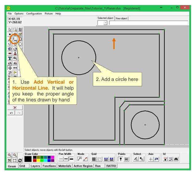
To draw the p-electrode and ppad we need to add several vertical and horizontal lines
