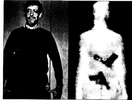
Millimeter wave detection of concealed weapon.
