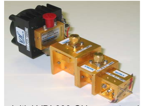
Initial VDI 600 GHz varactor chain Peak power 1.2 mW at 640 GHz
